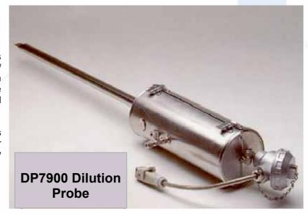
The dilution mechanism of the DP7900 probe is located outside of the stack, making the unit suitable for demanding applications including high temperatures (up to 1800 deg C), corrosive or exotic sampling environments, or stacks with a small internal diameter. The dilution probe is mounted using special quick release clamps for easy dismantling for filter checks and replacement.
