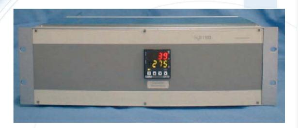
The Ecotech Model H<sub>2</sub>S-1100 Hydrogen Sulfide Converter employs both catalytic and thermal principles to convert H<sub>2</sub>S to SO<sub>2</sub>. Converter efficiency is better than 95% over a temperature range of 300°C to 400°C. (350°C is the optimal temperature for H<sub>2</sub>S conversion).
