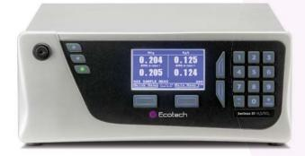
The Serinus® 51 analyser delivers precise and reliable performance at excellent value. It combines pulsed fluorescence detection with an internal catalytic converter to sequentially measure H<sub>2</sub>S and SO<sub>2</sub>in the range of 0 - 2 / 0 - 20 ppm respectively with a detection limit of 0.3 ppb.
